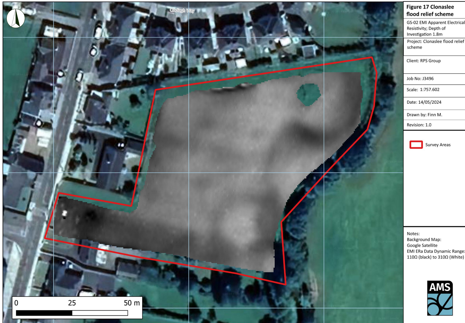
Figure 17. GS-02 EMI Apparent Electrical Resistivity; DOI 1.8m
