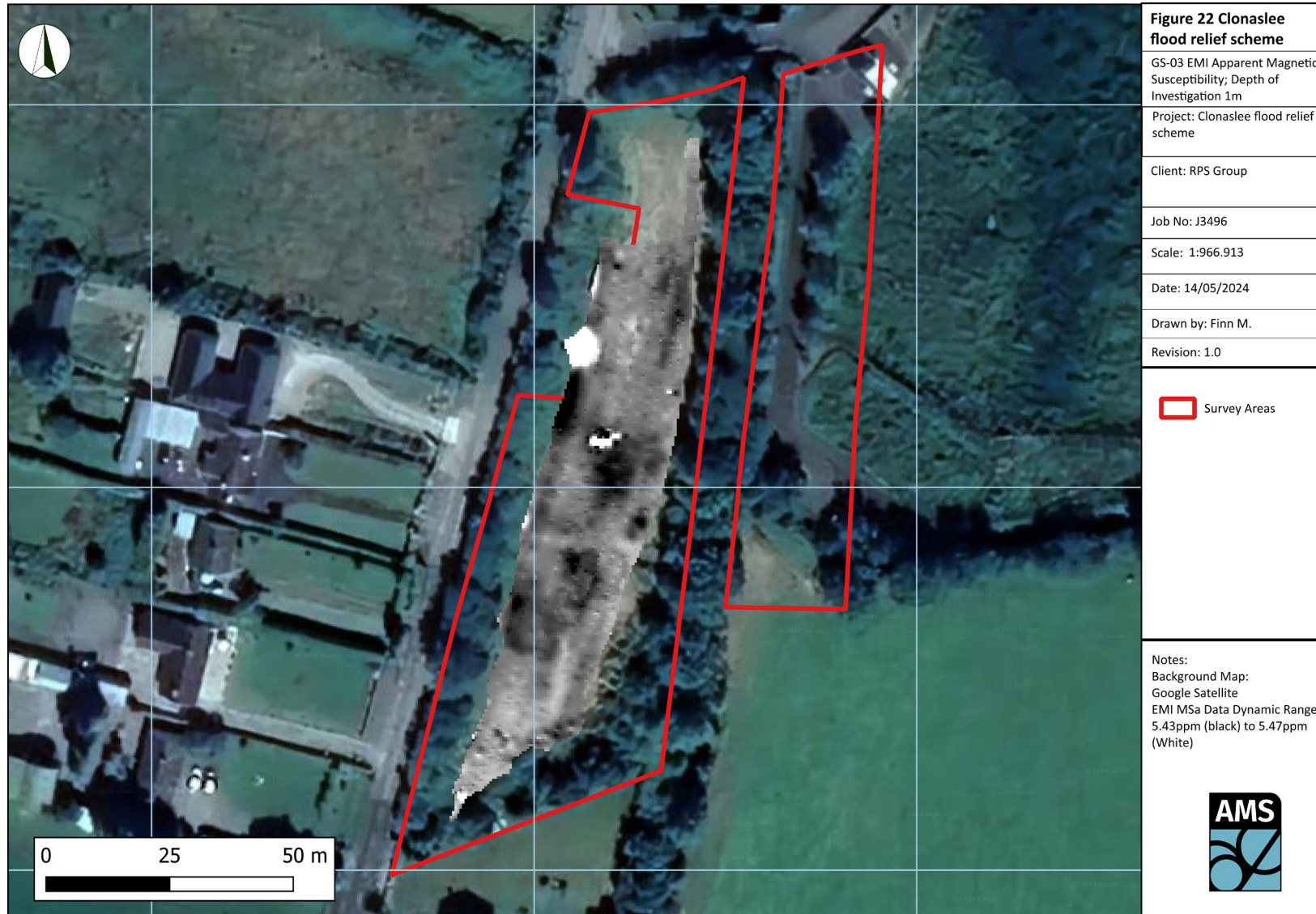
Figure 22. GS-03 EMI Apparent Magnetic Susceptibility; DOI 1m
