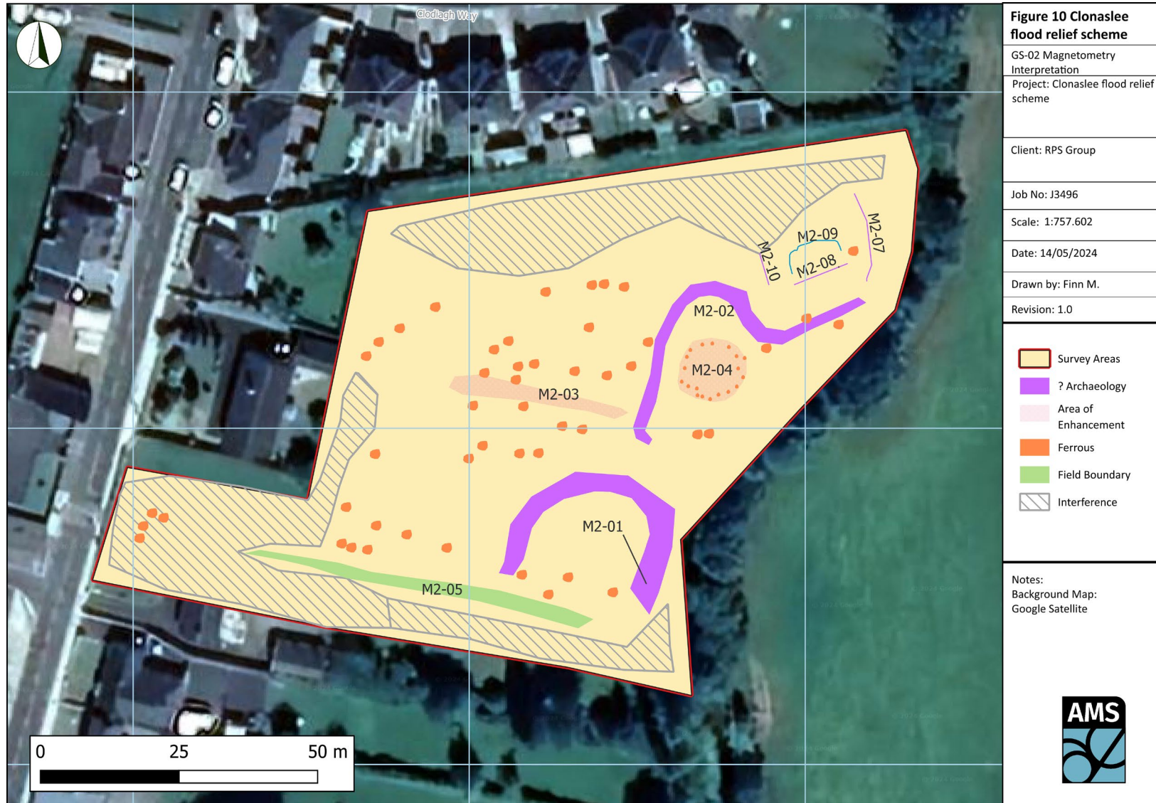
Figure 10. GS-02 Magnetometry Interpretation
