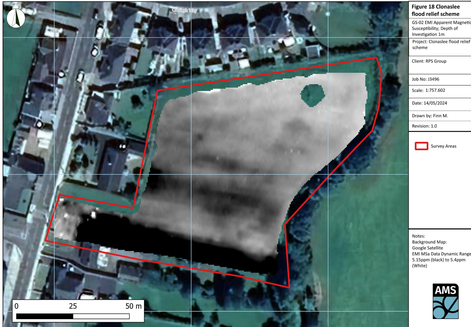
Figure 18. GS-02 EMI Apparent Magnetic Susceptibility; DOI 1m
