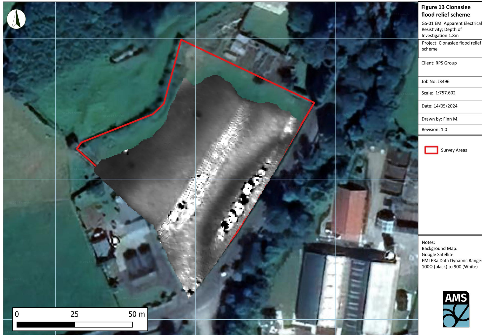
Figure 13. GS-01 EMI Apparent Electrical Resistivity; DOI 1.8m
