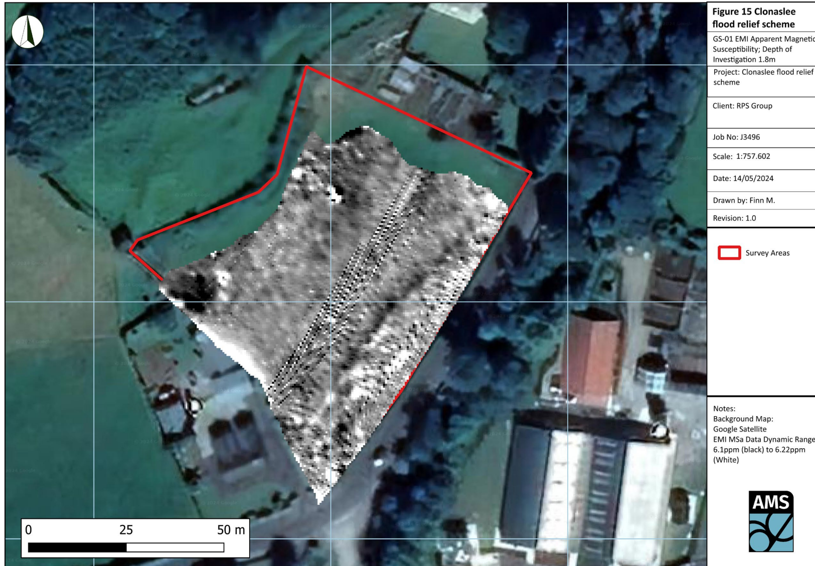
Figure 15. GS-01 EMI Apparent Magnetic Susceptibility; DOI 1.8m
