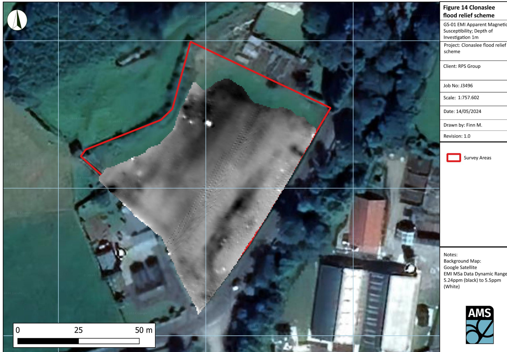
Figure 14. GS-01 EMI Apparent Magnetic Susceptibility; DOI 1m
