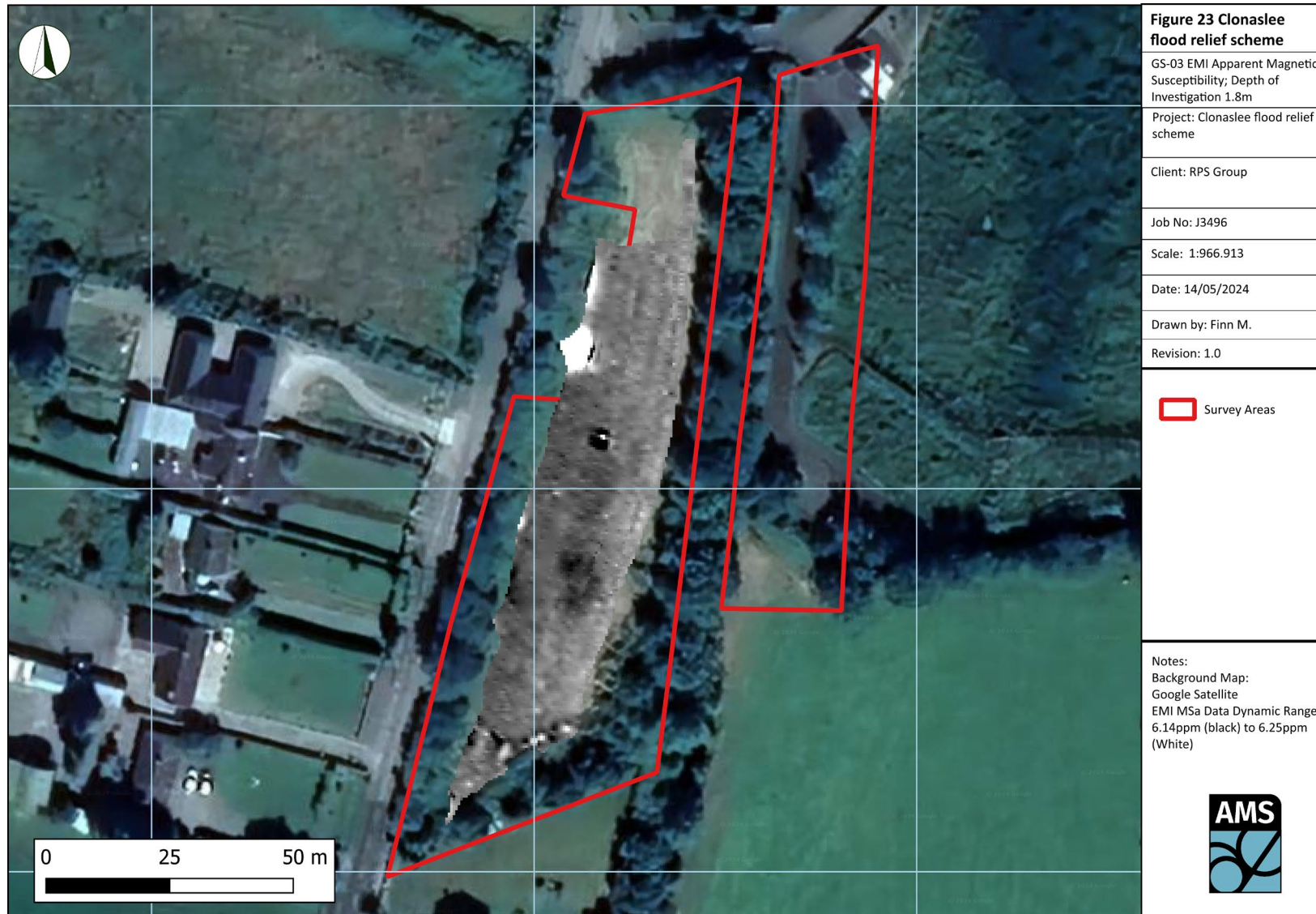
Figure 23. GS-03 EMI Apparent Magnetic Susceptibility; DOI 1.8m
