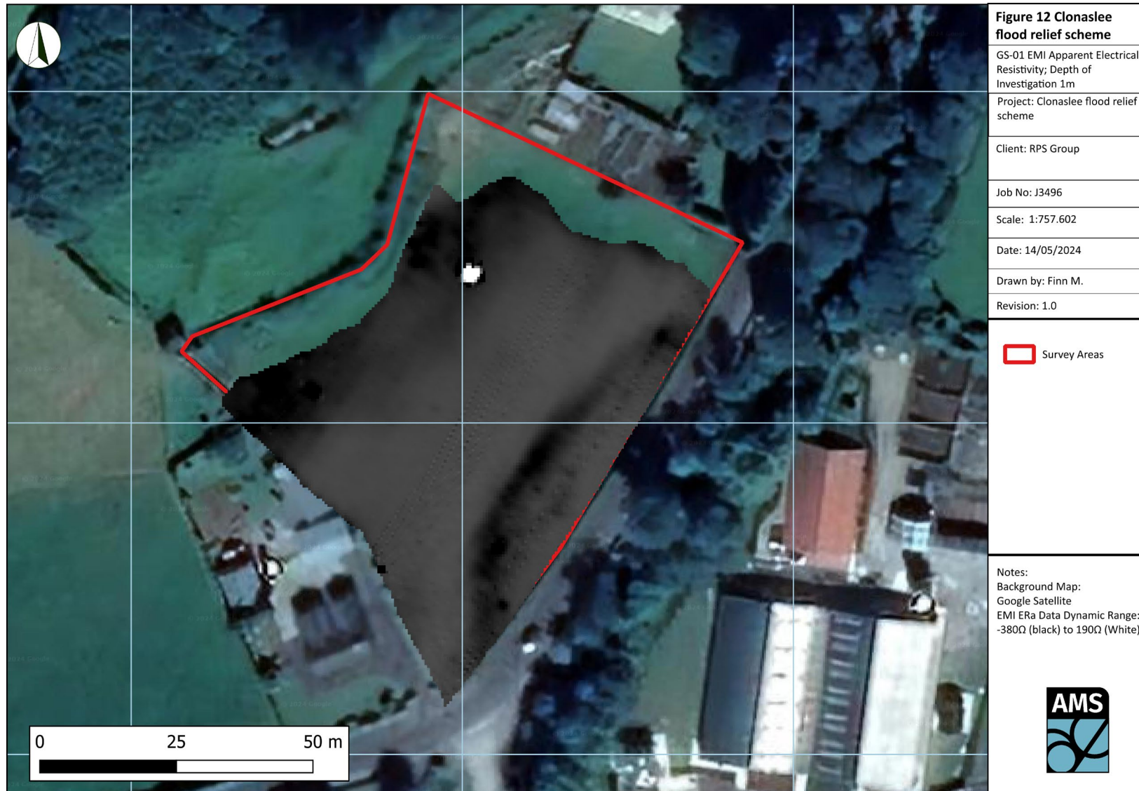
Figure 12. GS-01 EMI Apparent Electrical Resistivity; DOI 1m
