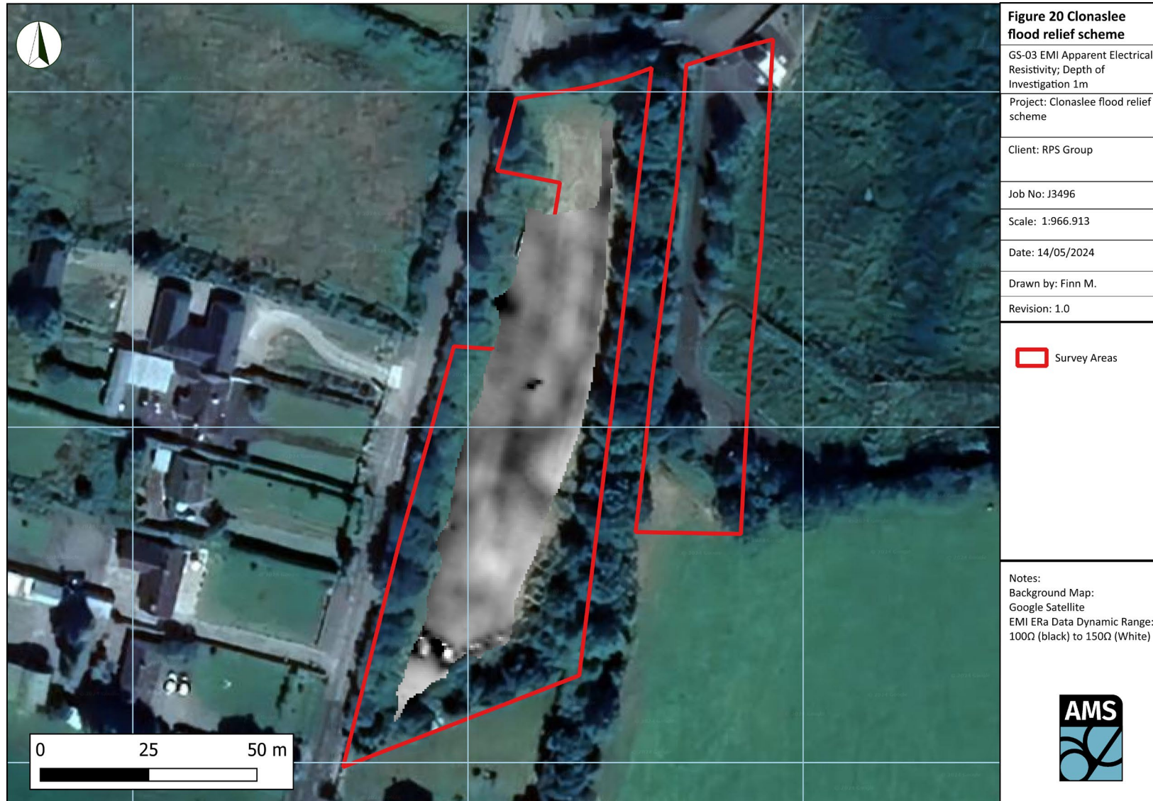
Figure 20. GS-03 EMI Apparent Electrical Resistivity; DOI 1m
