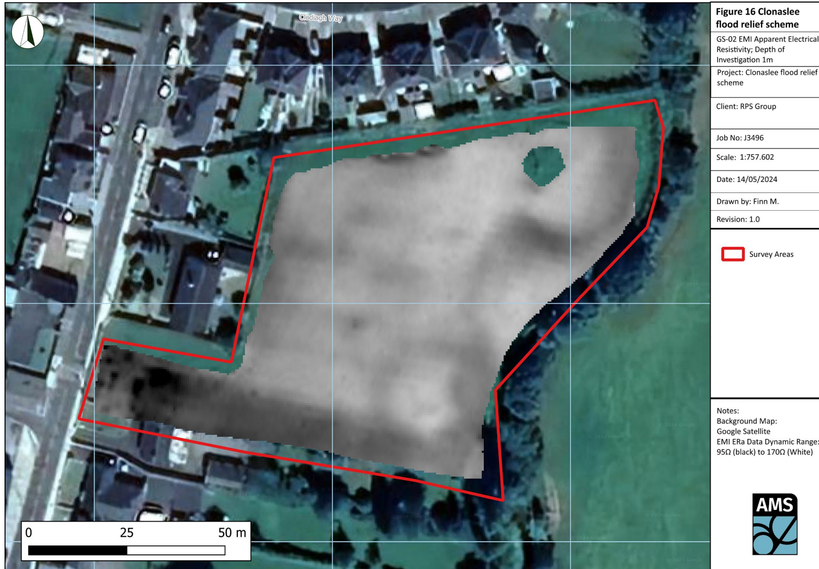
Figure 16. GS-02 EMI Apparent Electrical Resistivity; DOI 1m
