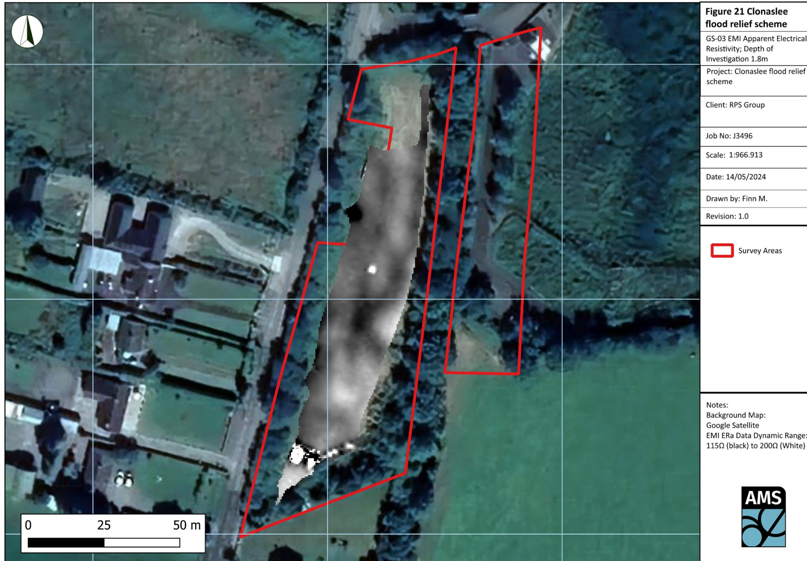
Figure 21. GS-03 EMI Apparent Electrical Resistivity; DOI 1.8m
